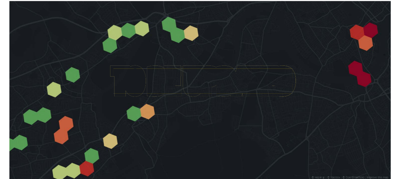
Figure 9 - Conceptual visualisation idea for national scale benzene and benzo(a)pyrene screening against GAC. Green denotes no GAC exceedances, with dark red indicating all locations within the hexagonal area having GAC exceedances.
